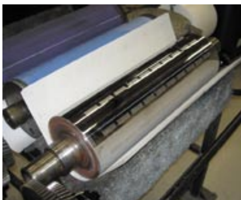
2.6 The strike-surface applying gravure roller, PC
