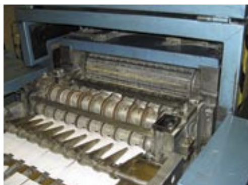
2.7 The machine that cuts the printed sheets longitudinally to the width of a matchbox, PC
