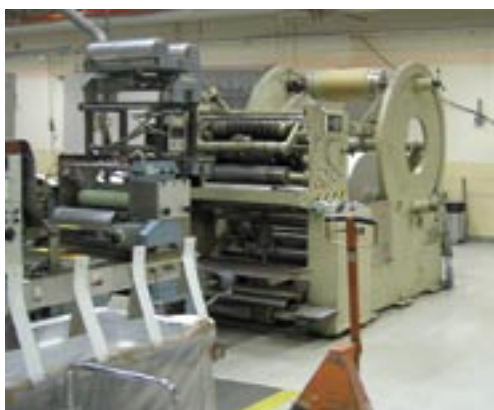
2.5 The reel-fed offset litho press, in this image, with an empty spool that holds the card to be printed, PC
